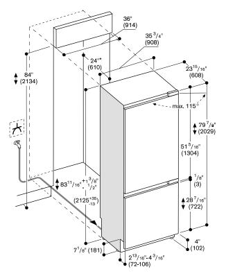
The door face dimensions are designed for a maximum gap of  $\mbox{\em 1/8}"$  (3 mm).
